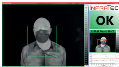
As soon as the test person enters the marked area (green field in the center of the image), the measurement starts
